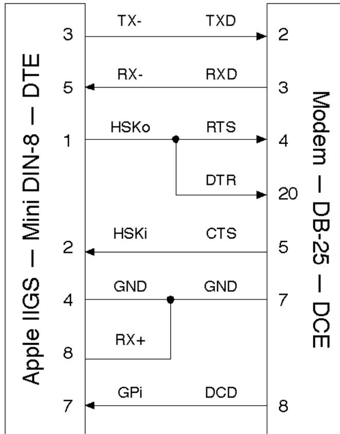
This cable provides true data carrier detection (DCD). It also supports hardware handshaking by connecting the Apple IIgs's two handshaking lines (HSKi and HSKo) to the modem's CTS and RTS lines. If hardware handshaking is not used, this wiring optionally supports DTR for disconnecting. The DTR wiring option is not required if the cable is to be used with only hardware handshaking.
